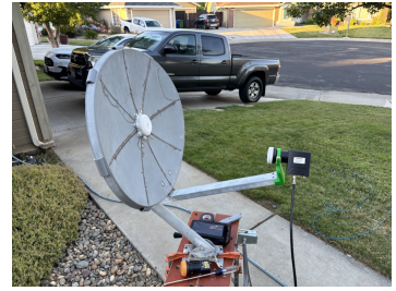
REPURPOSED DISH WITH GENERIC LNB
