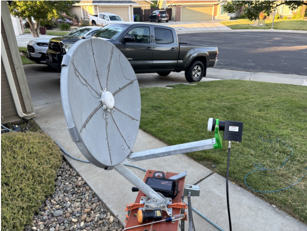
REPURPOSED DISH WITH GENERIC LNB
