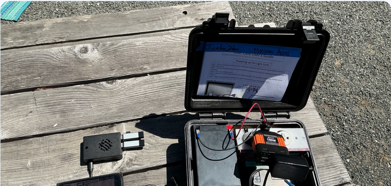
The complete kit: carry case, Raspberry Pi, power bank, and USB readers holding the language library cards.
